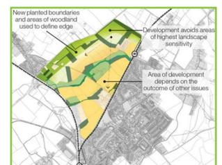
Issue 9: Response 3 - Diagram showing how the existing pattern of field boundaries and new areas of woodland and buffer planting can be used to create an appropriate edge to the expansion. Areas of higher ground are avoided to minimise visual impact.
