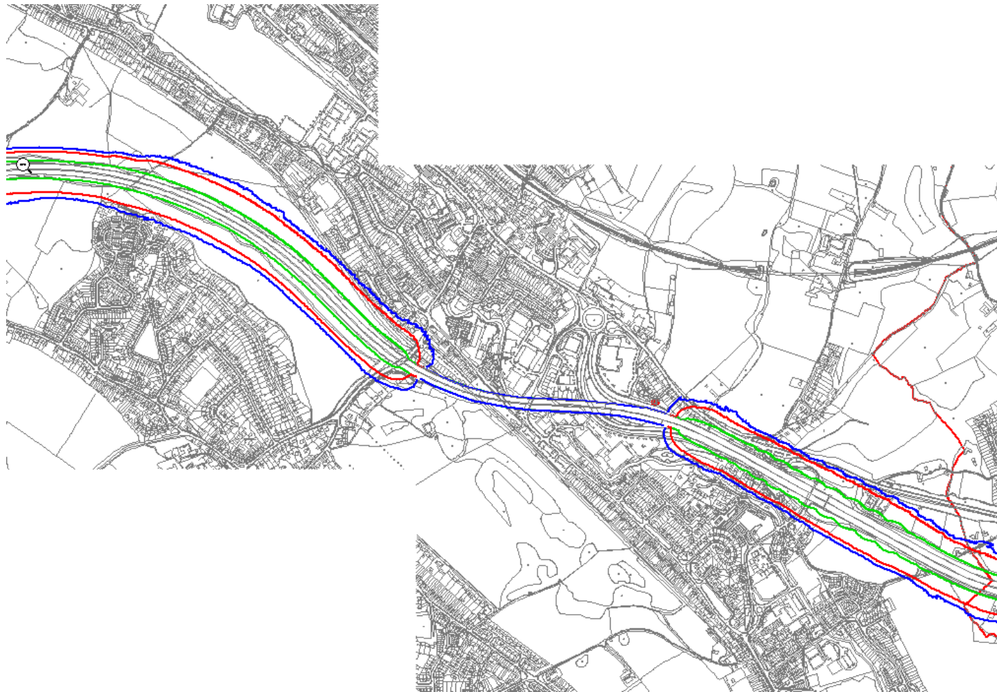
Figure 6 Modelled Annual Mean Nitrogen Dioxide Concentration Contours in 2009 along the M40 at the east end of the District (red dot is diffusion tube A). The red contour line represents 40 \mu\text{g}/\text{m}^3 , the blue contour line represents 36 \mu\text{g}/\text{m}^3 , and the green contour line represents 60 \mu\text{g}/\text{m}^3 . Contours stop at the elevated section of motorway. © Crown copyright 2010. All rights reserved, Wycombe DC. License number: 100023306
