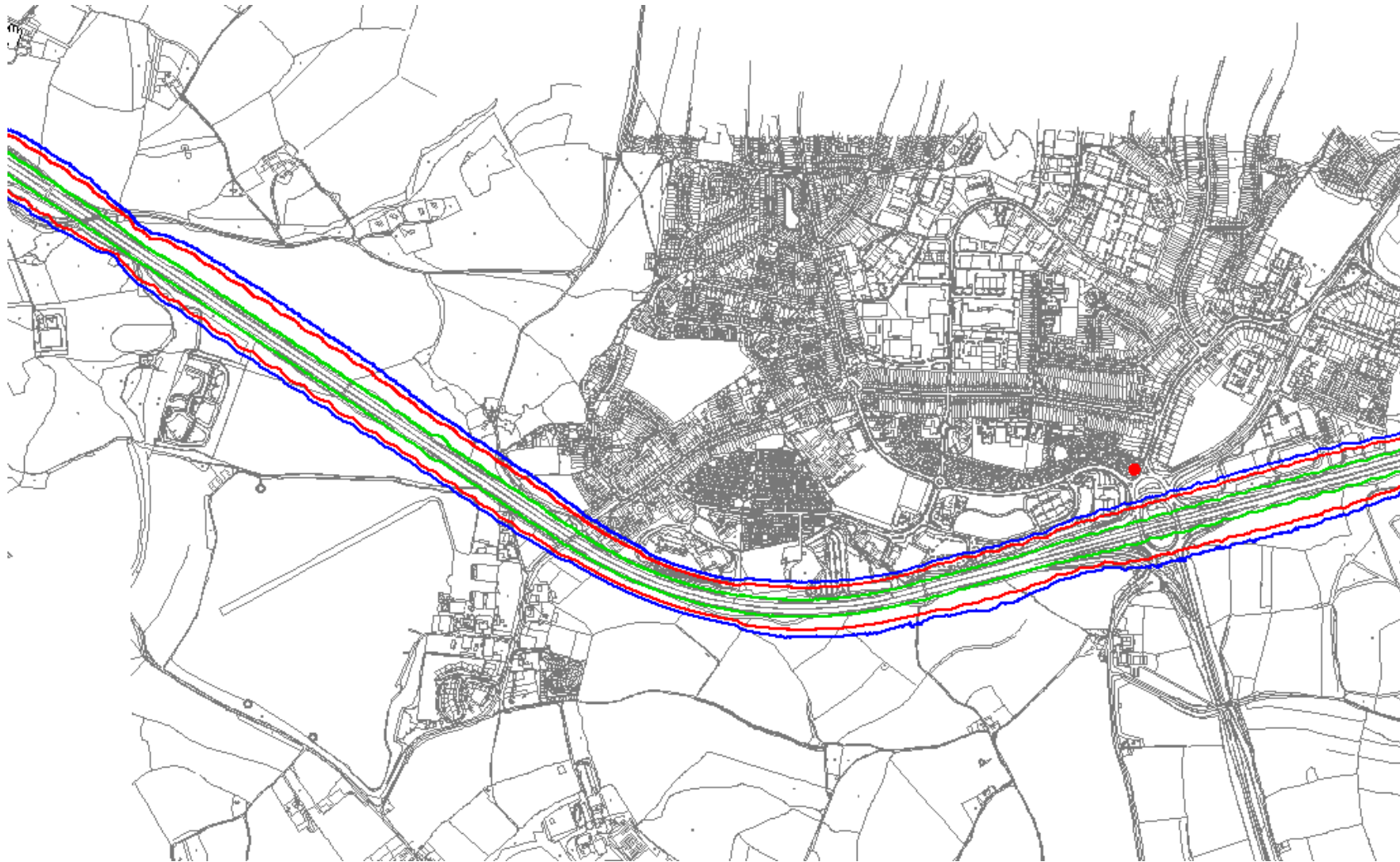
Figure 4 Modelled Annual Mean Nitrogen Dioxide Concentration Contours in 2009 along the M40 south of High Wycombe (red dot is diffusion tube H5). The red contour line represents 40 \mu\text{g}/\text{m}^3 , the blue contour line represents 36 \mu\text{g}/\text{m}^3 , and the green contour line represents 60 \mu\text{g}/\text{m}^3 . © Crown copyright 2010. All rights reserved, Wycombe DC. License number: 100023306
