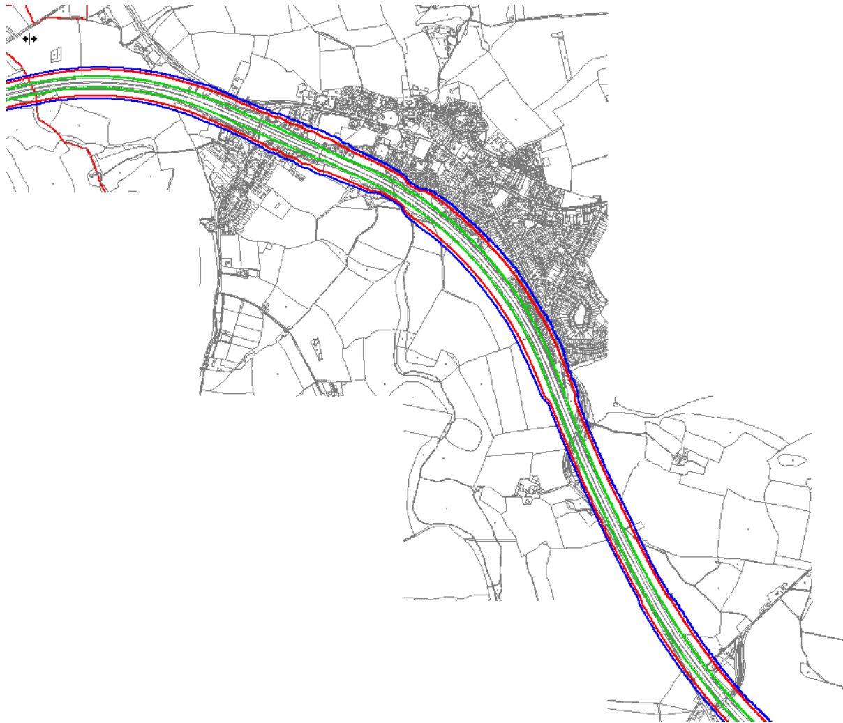
Figure 2 Modelled Annual Mean Nitrogen Dioxide Concentration Contours in 2009 within the west end of the study area (red line shows western boundary of Wycombe District Council). The red contour line represents 40 \mu\text{g}/\text{m}^3 , the blue contour line represents 36 \mu\text{g}/\text{m}^3 , and the green contour line represents 60 \mu\text{g}/\text{m}^3 . © Crown copyright 2010. All rights reserved, Wycombe DC. License number: 100023306
