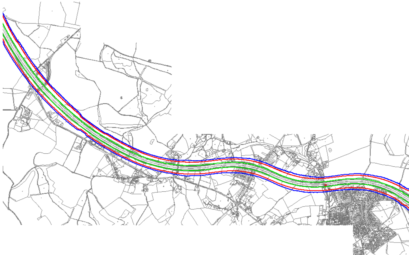
Figure 3 Modelled Annual Mean Nitrogen Dioxide Concentration Contours in 2009 along the M40 between Stokenchurch and High Wycombe (red dot is diffusion tube D). The red contour line represents 40 \mu\text{g}/\text{m}^3 , the blue contour line represents 36 \mu\text{g}/\text{m}^3 , and the green contour line represents 60 \mu\text{g}/\text{m}^3 . © Crown copyright 2010. All rights reserved, Wycombe DC. License number: 100023306
